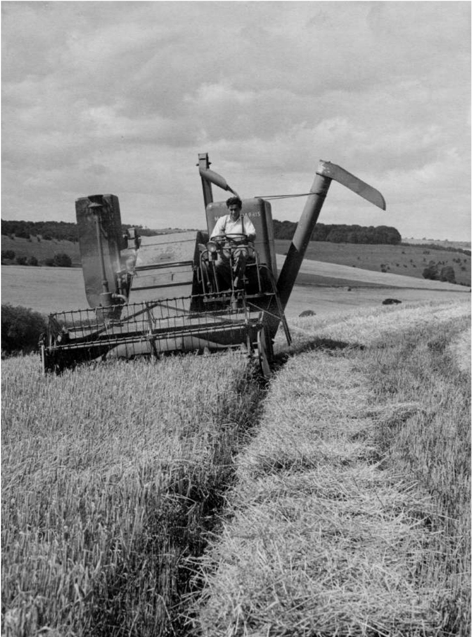
An early Massey Harris combine harvester. The first I had with onboard bulk tank facilities for grain collection. Prior to this, the corn had to be put into sacks and manually handled.
